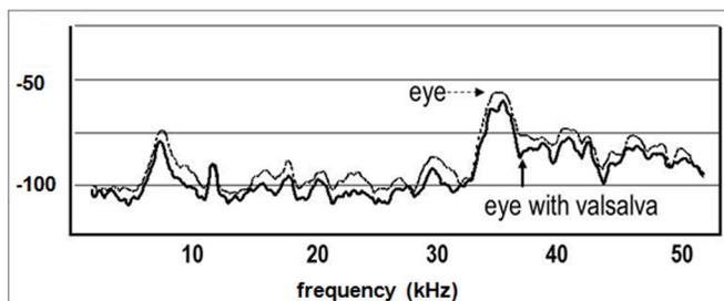
**Figure 4.** In one subject, vibration response of the eye induced by broadband noise delivered to the head. With pressurization (Valsalva maneuver), the vibratory response is damped over a wide frequency range by 4–6 dB (re: 1 volt). The natural resonance of the eye is approximately 35 kHz, with subharmonic peaks.
