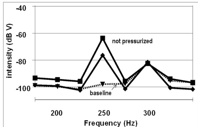
**Figure 3.** Vibratory response of the eye balloon with and without (baseline) forced vibration of the skull at 250 Hz. With pressurization, the response at the skull driving frequency (250 Hz) is damped by 12 dB (re: 1 volt).
