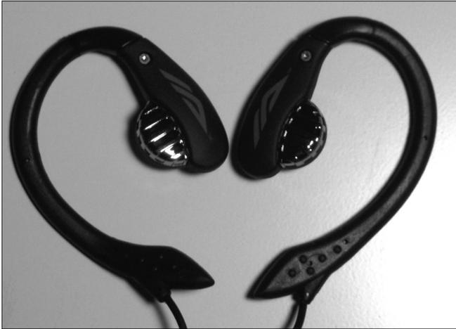
**Figure 1.** AirDrives Interactive Stereo earphones: the speaker sits outside of the ear and transmits sound via the tragal cartilage.
