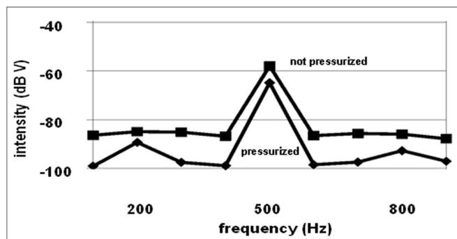
**Figure 2.** Vibratory response of the eye balloon as a function of frequency using a forced vibration of 500 Hz delivered by a vibrator on the skull. With pressurization of the balloon brain, the eye response is damped 7 dB (re: 1 volt).
