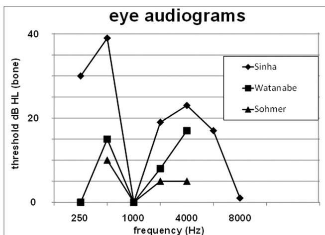
**Figure 5.** Eye audiograms as a function of bone conduction hearing level and frequency for five subjects (Sinha), contrasted to the data of Watanabe et al.<sup>15</sup> and Sohmer et al.<sup>12–14</sup>. Other than the ambient low-frequency noise masking in the Sinha data, the plots are in good agreement, with maximal sensitivity at 1,000 Hz. The eye is as sensitive as the skull, opening up the possibility of another method of stimulating the inner ear through a fluid conduction mechanism.
