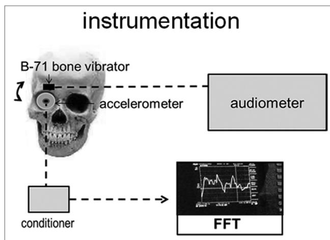
**Figure 1.** Instrumentation used in the study. Sounds were generated by an audiometer and delivered to either the skull or the eye (in the model) or, for the hearing tests, to the eye using a standard clinical bone conduction vibrator. Vibration of the balloon eye was recorded by a piezoelectric accelerometer, amplified and conditioned, and fed into a fast Fourier transform (FFT) for analysis.
