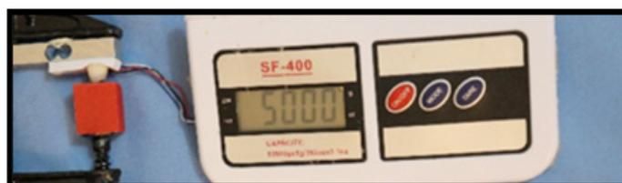
Figure 3: Customized loading device (5000 g).
