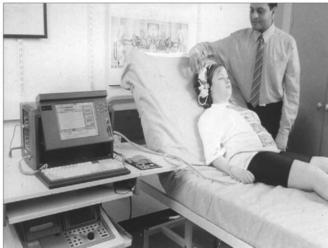
**Figure 1.** The Southampton Tympanic Membrane Displacement (TMD) Analyser. Patient reclining on a bed, supine in a 45-degree position for recording of IPPA. A recording probe in place in the right ear canal and maintained with a head band. The doctor is standing to the patient's left. The equipment is in two boxes.
